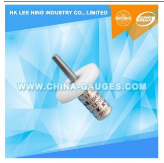
The Test Pin (**Figure 2B of IEC 60950**) is intended to verify the protection against access to hazardous live parts in class 0 equipment and class II equipment.
