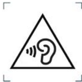
Figure Z1 – Warning label (IEC 60417-6044)
