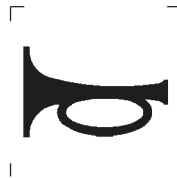
Figure F.3 — Electric horn symbol
